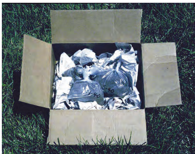
Figure 15.14. Soil samples prepared for shipping or transport to the lab, in a cardboard box cushioned with newspaper to reduce drying, heating, and rough treatment, which can damage the nematodes and interfere with the lab's ability to recover them.
