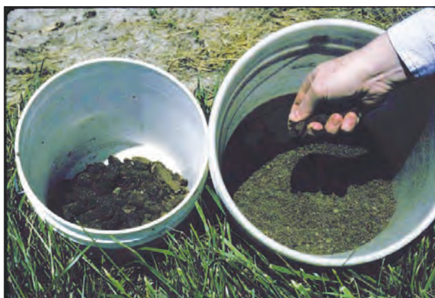
Figure 15.13. After all cores are collected for a sample (left), the soil should be mixed gently but thoroughly (right).
