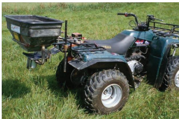
Figure 6.2. Spinner-type seeder for frost seeding mounted on an all-terrain vehicle.
