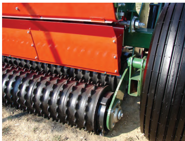
Figure 6.4. Double-corrugated roller-seeder (Brillion brand).
